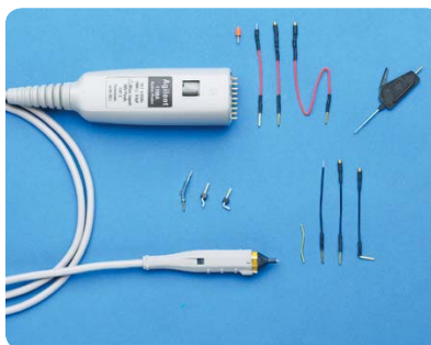
Agilent 1156A active probe with accessories
