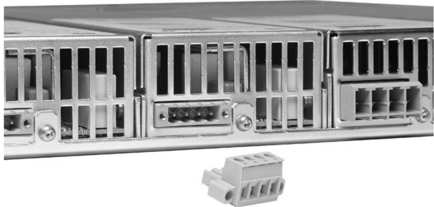
Figure 5. Quick disconnects for power and sense leads
