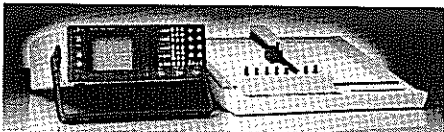
The PM 3350 can directly drive plotters thru the IEEE-488 or RS 232 interfaces. Hard copies can also be made using standard dot-matrix printers.
