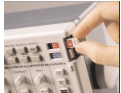
Application Module being installed.
