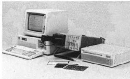
DCS01 Digitizing Camera System captures repetitive waveforms from analog scopes and transients according to a scope's CRT writing speed (400 MHz for 2467B).
