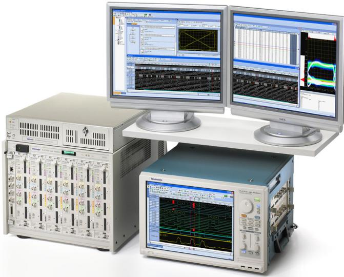
The modular TLA7000 logic analyzer series provides the speed and flexibility you need to capture logic detail on today's fastest designs. Pinpoint the source of elusive errors and gain the visibility you want with large easy-to-read displays, fast data throughput, and time-correlated views of analog and digital signals through the same probe.
